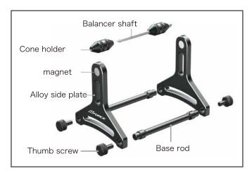
Carefully install the wheel balancer as illustrated. The logo on side plates must face out. The magnets must be positioned so they attract, not repel.
