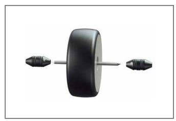
Fit the wheel to shaft and push the cone holders to wheel firmly. The cone holder is designed for different types of wheels. One side is make Φ4 is for metric type of wheels and other is for imperial.
