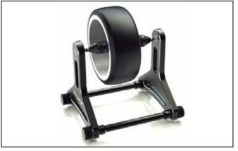
The principle of balancing is to find the "heavy side" of a wheel and add weight to the light side. Using your finger to spin the wheel and it will come to stop with the "heavy spot" at the bottom. Apply weight to opposite. A wheel is perfectly balanced if it can be stopped and will remain stationary in any position. Balance wheel will make big difference in the smoothness and handling of your car.
